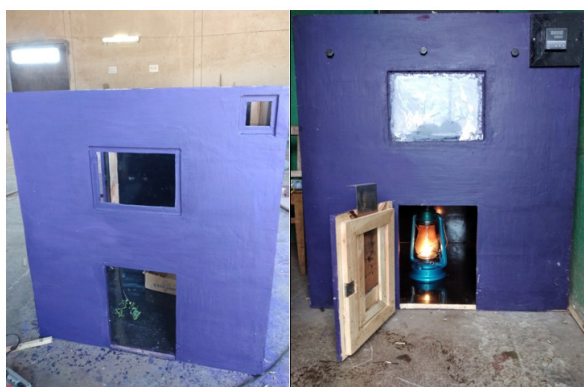
Figure 1: Prototype of electric and kerosene lump egg incubator
