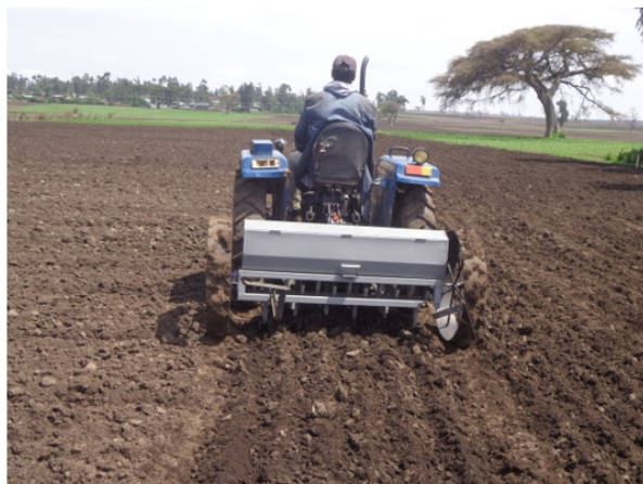
Figure 1: Field performance evaluation of seed drill Laboratory performance test Mechanical
