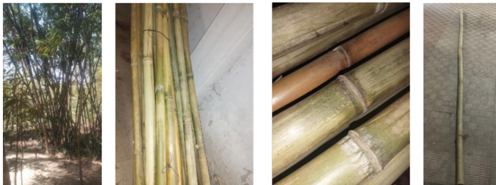
Figure 6: (From left to right) The source of the bamboo Culm; storage of the bamboo; Mitinga shows mature strong node at 700-900mm distance; Relatively straight, large internodal distance Source: Author
