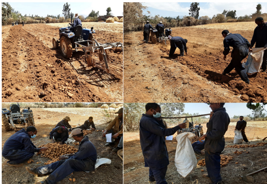
Figure 2: Data collection during performance evaluation of tractor-drawn potato digger
