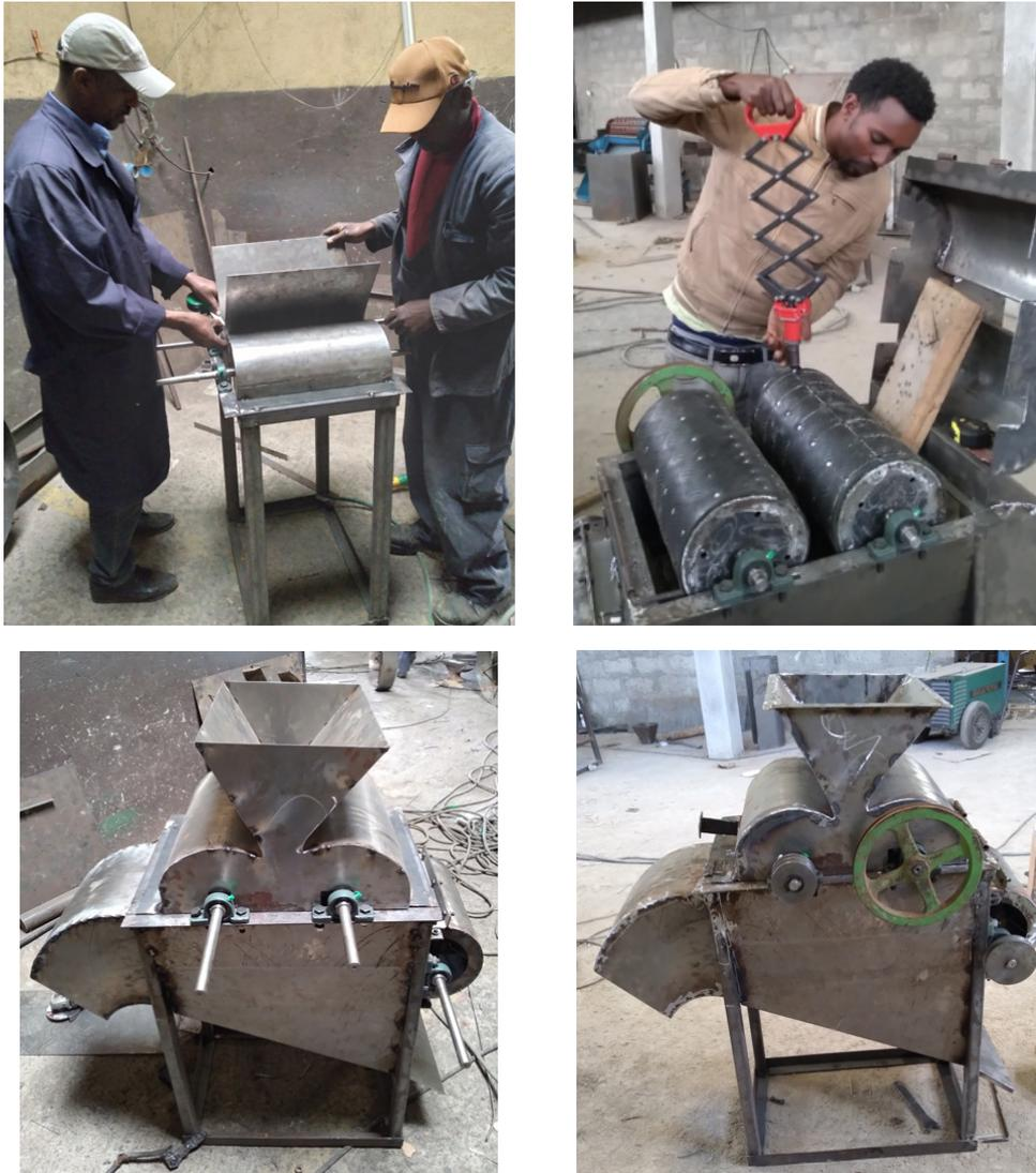
Figure 20: Prototype construction of garlic bub breaker
