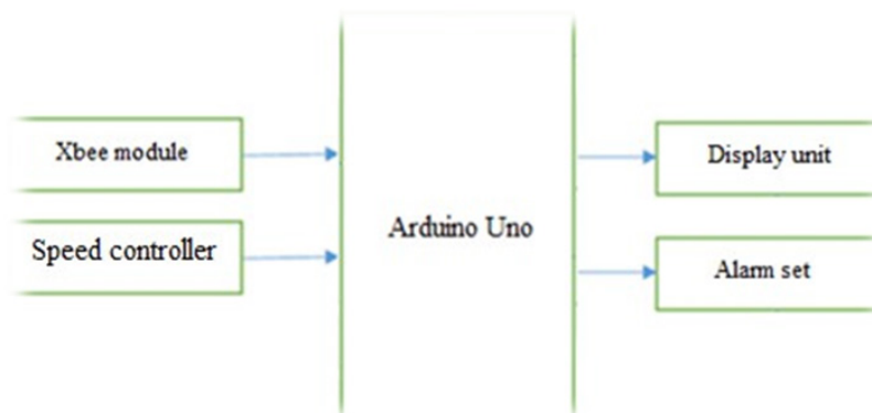
Figure 2: Receiver block diagram
