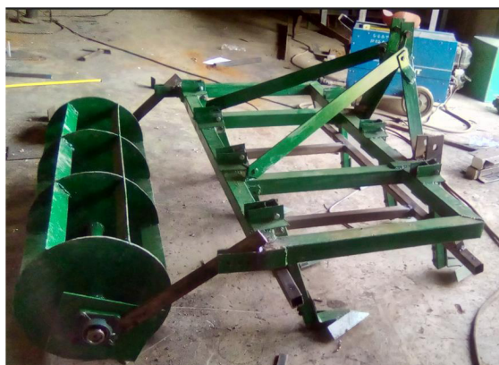
Figure 3: Prototype Cultivator with Pulverizing Attachment after Fabrication and during Testing
