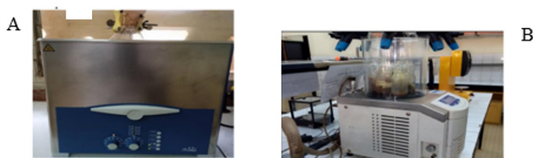
Figure 2: The Clifton Range Ultrasonic bath (A) Laboratory freeze dryer Alpha 1-2 LSCbasic (B);
