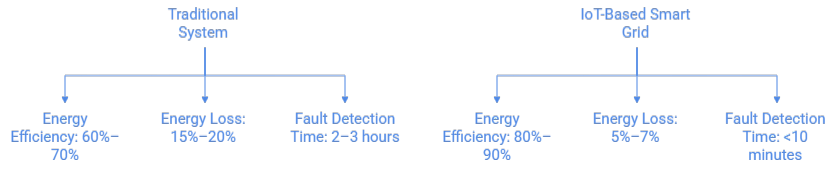
Figure 6: Comparison of Traditional and IoT-Based Smart Grids
