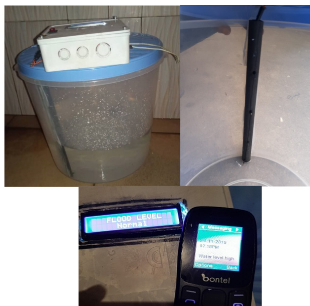
Figure 15: Complete Flood Detector System
