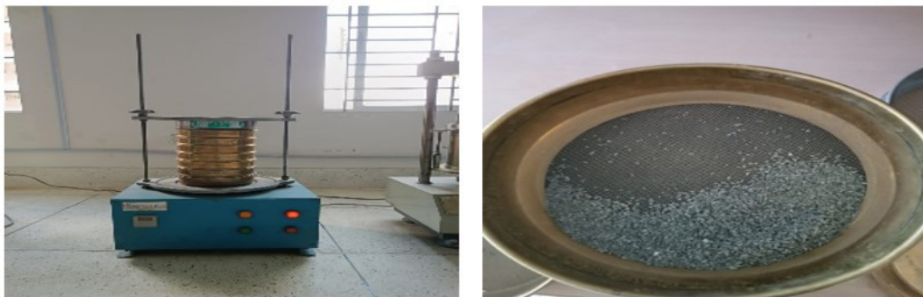
Figure 6: Photograph of procedure of fine aggregate grading test
