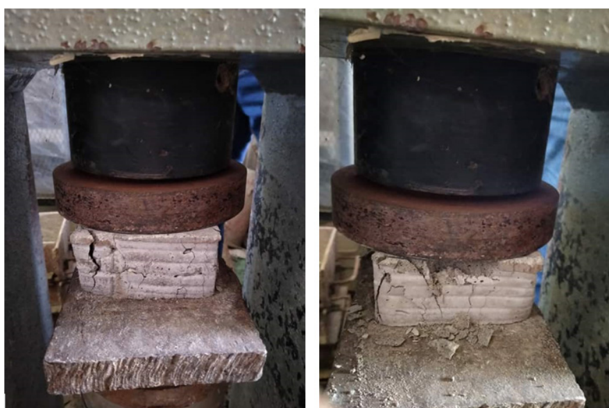
Figure 2: Specimens subjected to the Universal Testing Machine (UTM)
