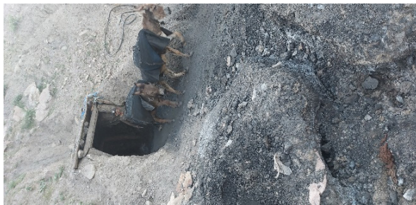
Figure 4: Primitive Transportation of Coal from Informal Shafts in the Shindarah Coal-Bearing Area
