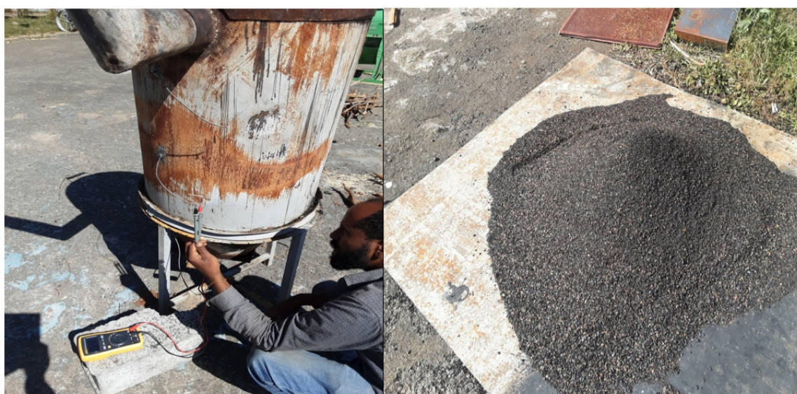
Figure 2: Carbonizer prototype during performance testing
