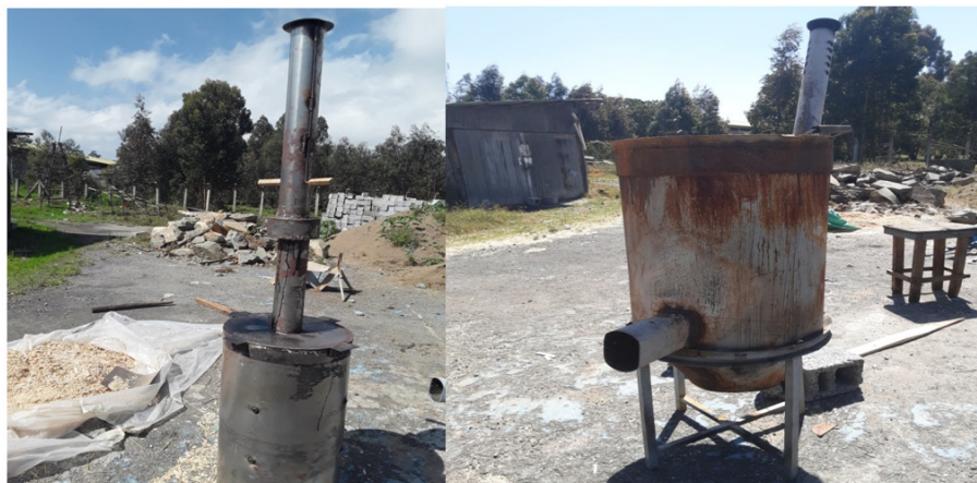
Figure 1: a) BAECR corncob-type Carbonizer, b) JAERC Closed drum-type carbonizer
