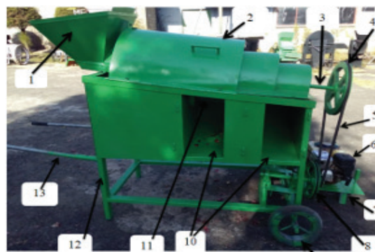
Figure 1: Pictorial view of the fabricated onion grading machine prototype.
