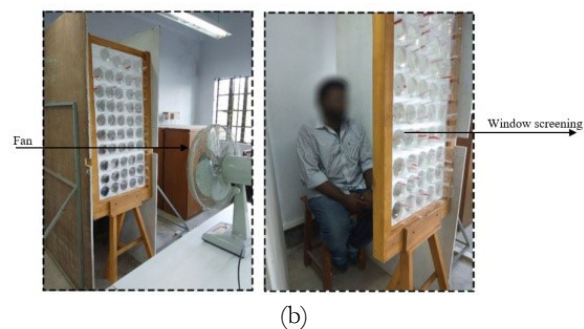
Figure 1: (a) Experimental chamber and (b) experimental setup with the subject (bottom right)
