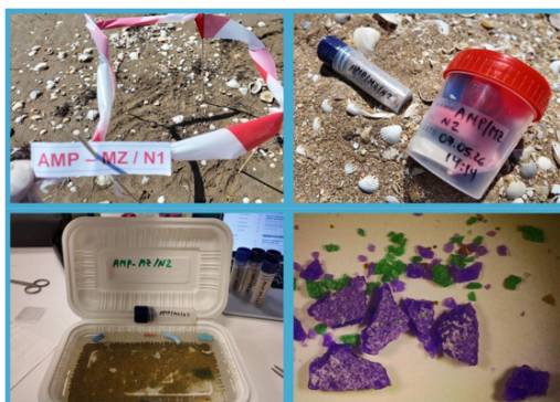
Figure 2: Field sampling, sample coding and saltwater flotation stages in Absheron National Park and Zira.
