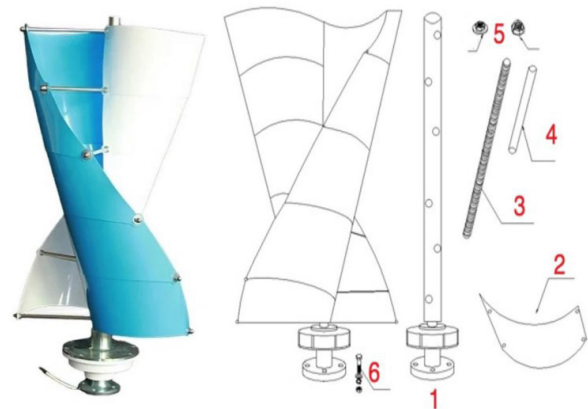
Figure 4: Savonius Vertical Axis Wind Turbine
