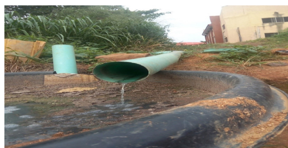
Figure 1: Raw Grey-water from Jadesola Akande Hostel to the Sedimentation tank at the Experimental Field
