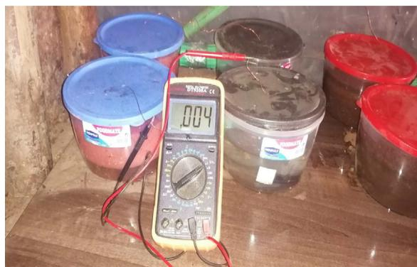
**Figure 1.** Set-up of H-shaped microbial fuel cells with a multi-meter
