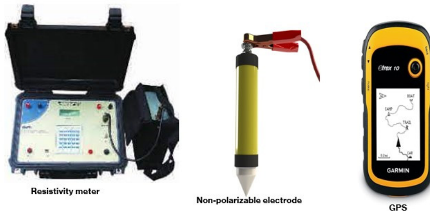
Figure 3: The basic instruments used in the field survey
