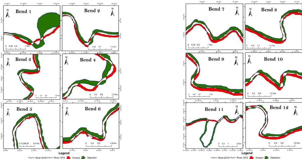
**Figure 2:** Erosion and Deposition in bend 1-12 from 1972-2016
