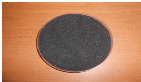
Figure B: Activated Carbon Derived from Bark of BM 5g/l at 350°C and the residual concentration is measured the usage atomic absorption spectrophotometer.
