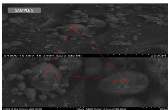
**Figure 4:** SEM images of unheated raw fly ash at three different magnifications
