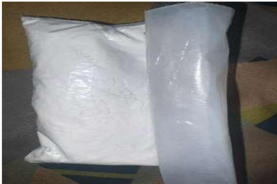
Figure 1: RHA-derived nano-silica powder produced for this study (author's fieldwork, 2026).
