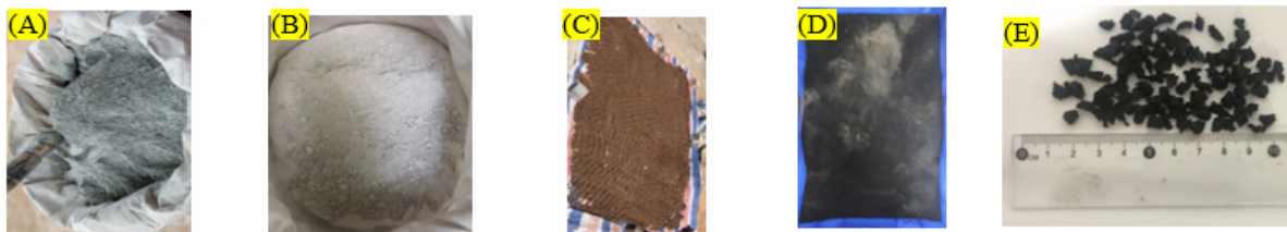
Figure 1: materials used in this study: (A) OPC binder; (B) SLAG binder; (C) Natural FA (Sand); (D) CR as binder materials and; (E) CR as FA
