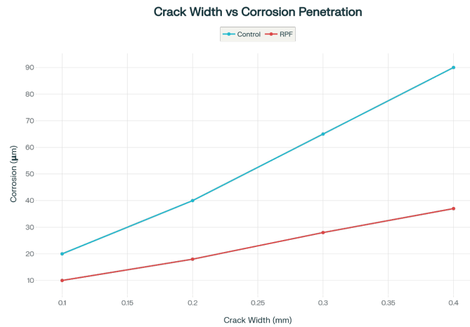
Figure 6: Crack Width vs. Corrosion Penetration for RPF and Control Concrete
