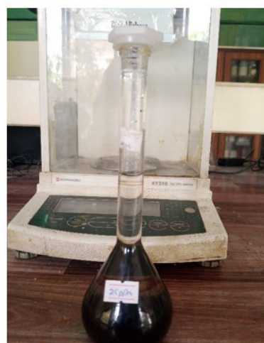
Figure 4: Preparation of Cr(VI) Stock Solution Using Potassium Dichromate ( K_2Cr_2O_7 )
