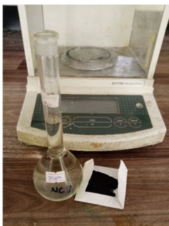
Figure 3: Experimental Setup for Adsorbent and Chromium Solution Preparation
