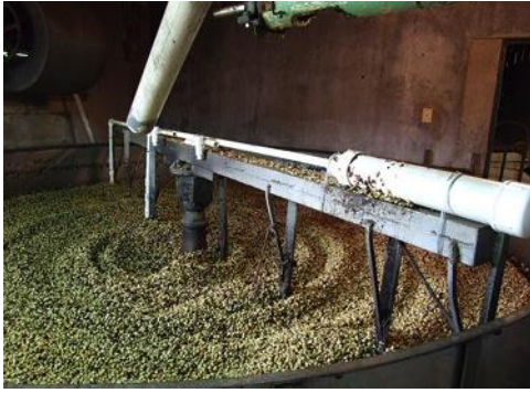
Figure 1: Depiction of a typical rotary drum drier (batea) used in Puerto Rico to dehydrate parchment coffee ( C. arabica ). This particular batea was instrumented to collect coffee mass and air data in situ for typical drying cycles.
