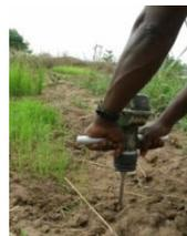
**Manual Cone penetrometer in use**
