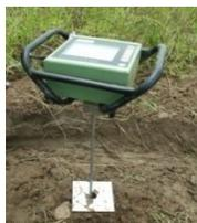
**FIG. 1: Digital Cone penetrometer**
