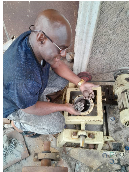
Figure 1: Crushing the raw materials using a locally-made ball mill
